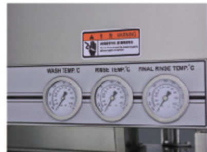
Reliable mechanical type thermal control and temperature gauges.
